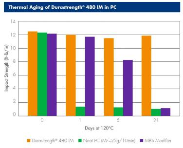
\*ASTM D256 specifications for notched IZOD impact tests.
